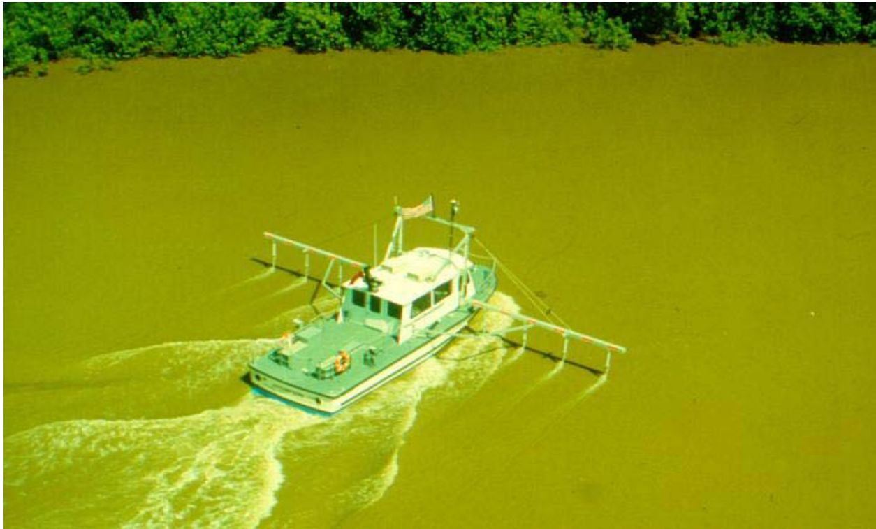
Figure 10-2. Typical Ross boom sweep system (St. Louis District)
