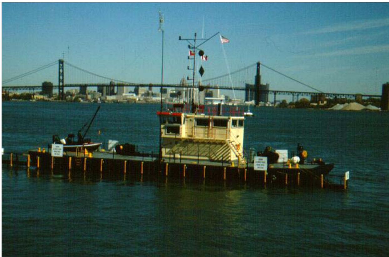
Figure 10-5. Detroit District Survey Vessel PAJ, a 120-ft, 32-channel sweep system
