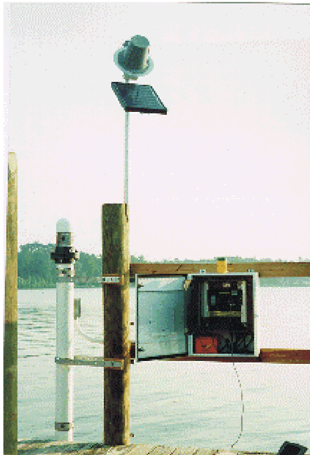
Figure 5-13. Primary automatic gage to record tides
