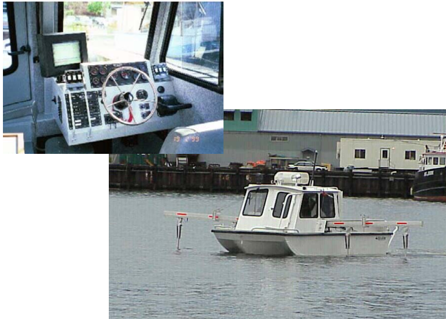
Figure 10-6. St. Paul District Five-Channel Ross Mini Sweep System
