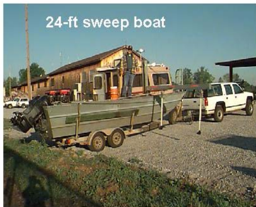
Figure 10-7. Mobile District (Tuscaloosa Site Office) sweep vessels
