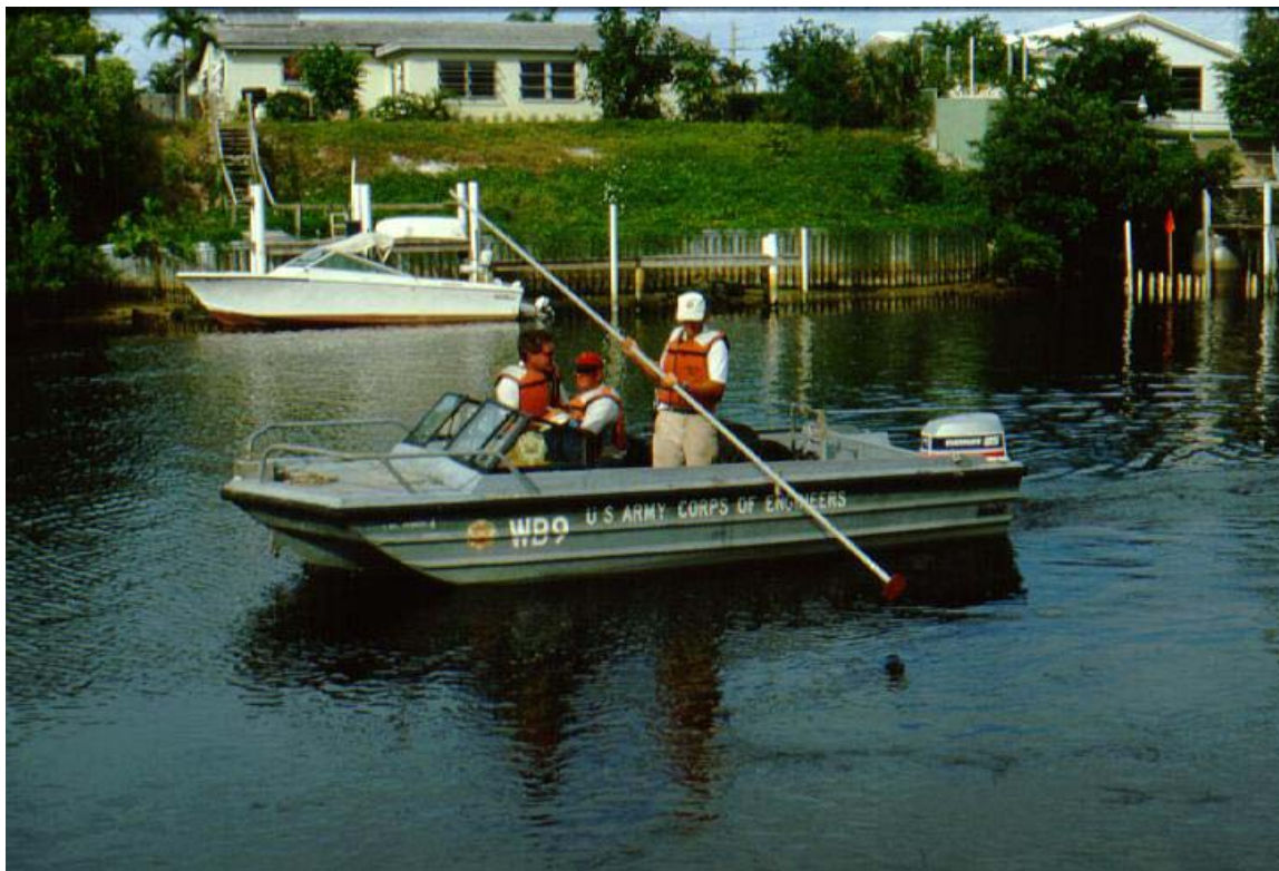
Figure 8-4. Sounding pole measurement from small work boat (Jacksonville District)
