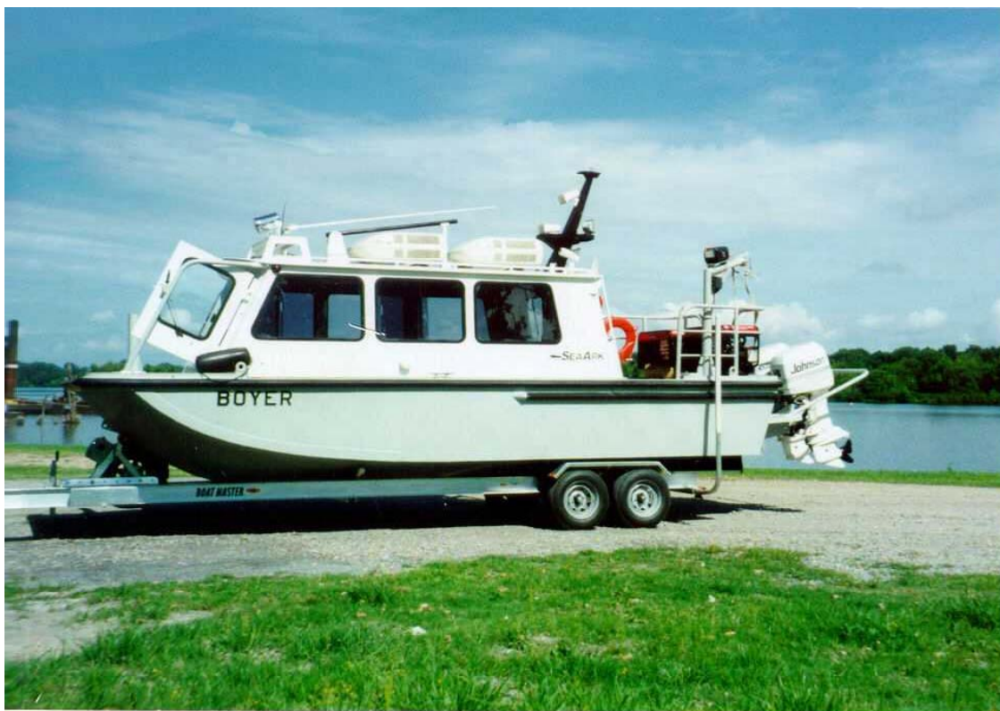
Figure 6-2. Corps standard trailable survey boat with twin outboard engines and enclosed work cabin (Surveyboat Boyer, St. Louis District)
