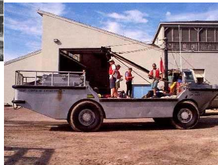
Figure 18-7. Sled profiling system--LARC with towed sled. Used to collect profile data through the surf zone and into the nearshore areas
