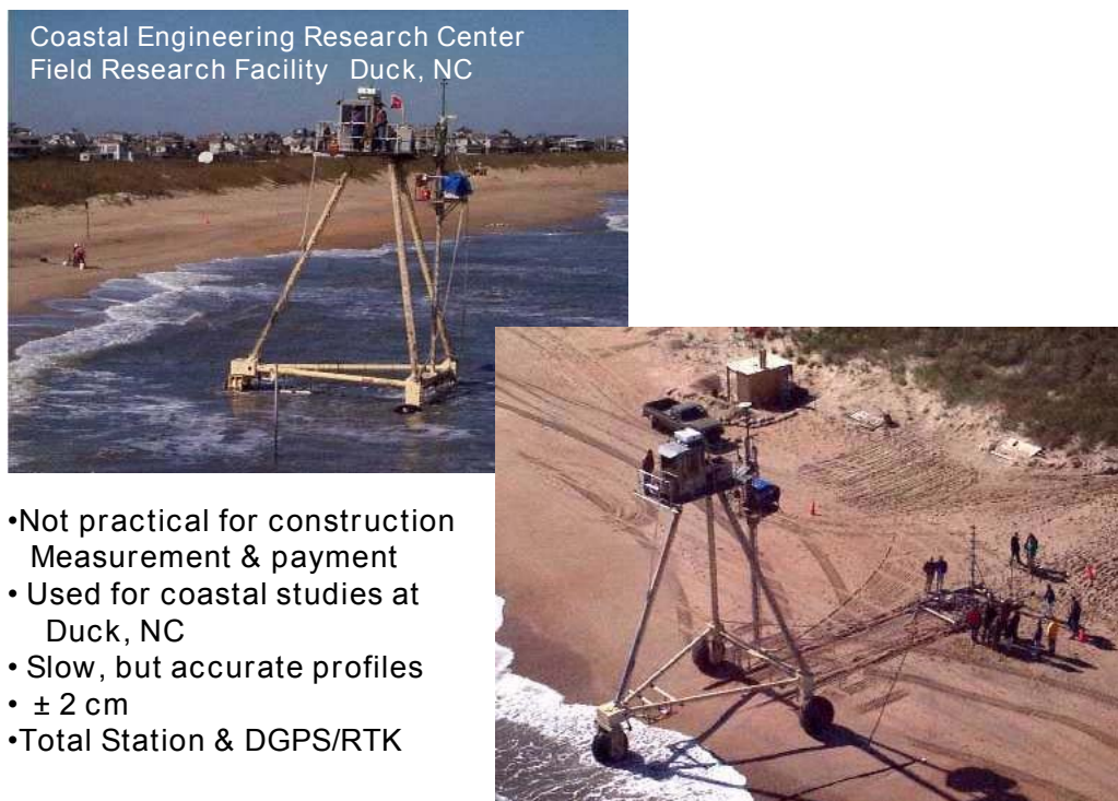
Figure 18-6. CRAB. Hydrographic survey platform used for research purposes by the Coastal Engineering Research Center (Duck, NC)
