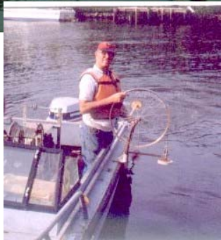
Figure 8-2. Lead line measurements (Jacksonville District)
