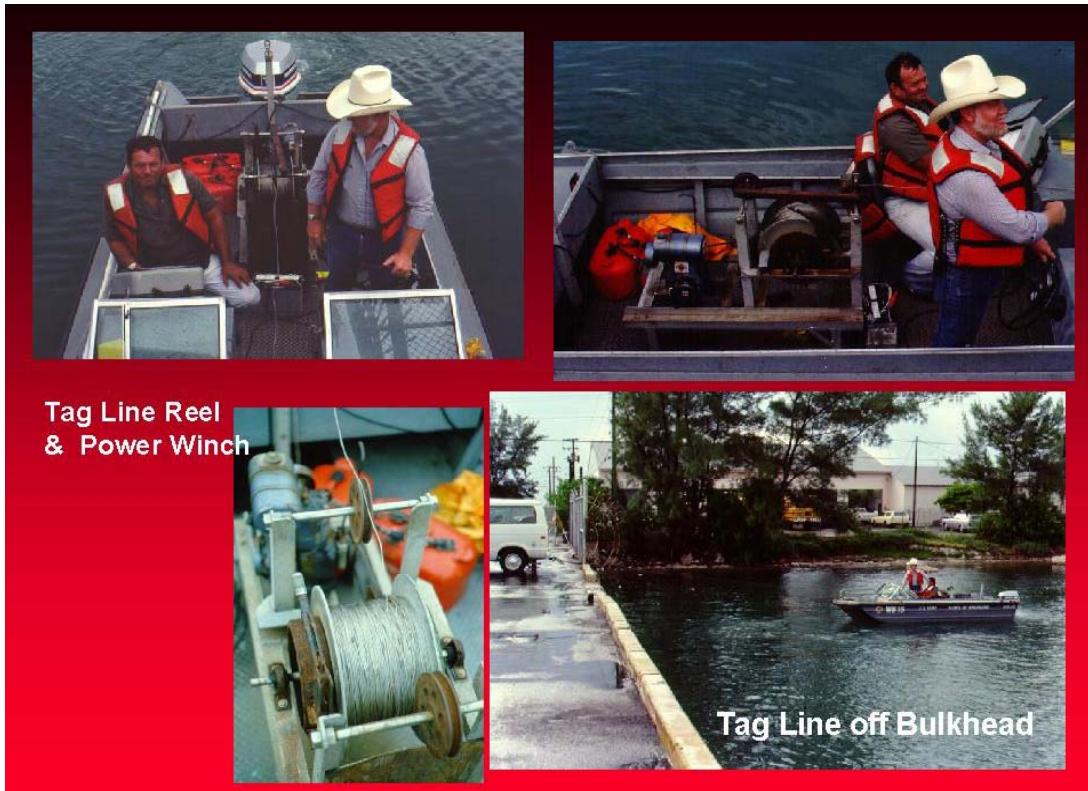
Figure 7-10. Tag line equipment aboard small 19-ft workboat (Jacksonville District)
