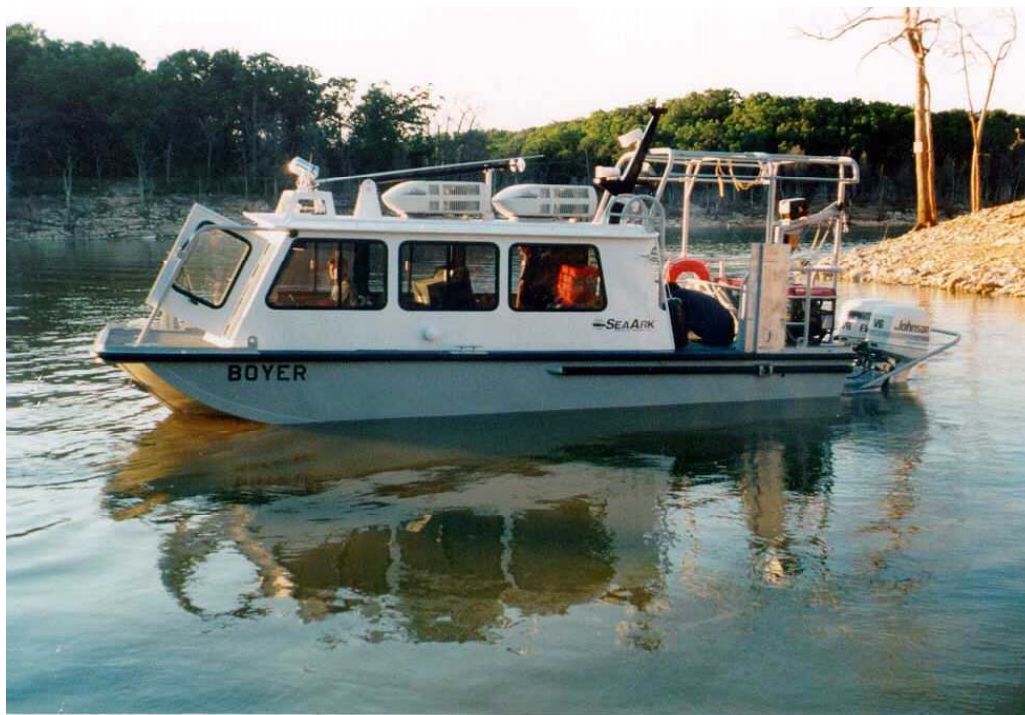
Figure 17-6. MV Boyer (St. Louis District) -- used for river engineering surveys and investigations on the Middle and Lower Mississippi River
