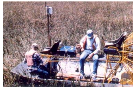
Figure 8-2. Lead line measurements (Jacksonville District)
