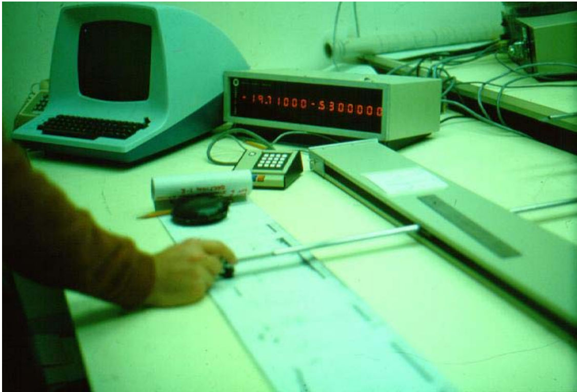
Figure 15-5. Automated quantity take-offs from digitizing tablet (ca 1976 Jacksonville District)
