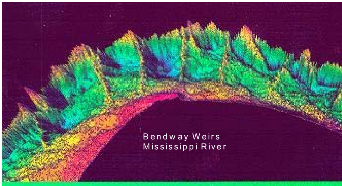
Figure 17-7. Bendway weir multibeam surveys (St. Louis District)
