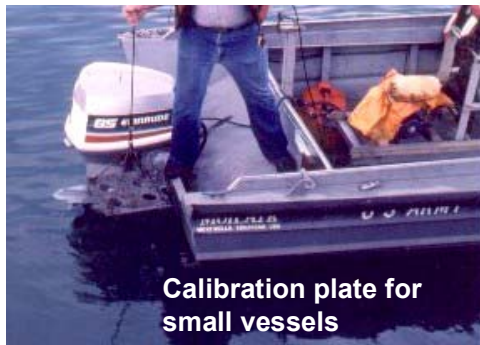
Figure 9-9. Bar check calibration (Jacksonville District)
