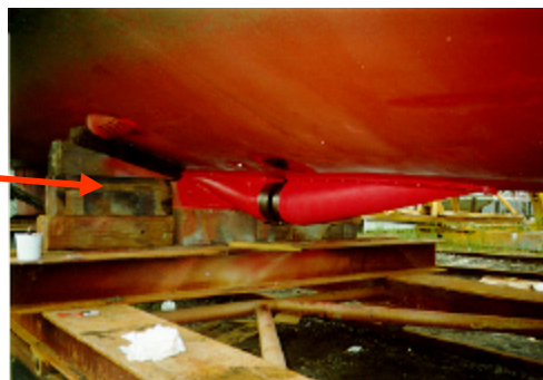
Figure 11-7. RESON SeaBat 8101 installation on Survey Vessel Adams II (Norfolk District)
