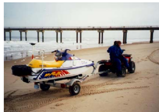
Figure 18-9. Yamaha Wave Runner equipped with hydrographic survey equipment (SCAMP at Duck, NC)
