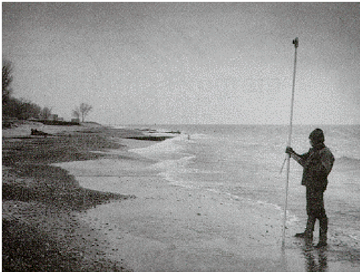
Figure 18-5. Rod and transit beach surveying provides accurate beach profiles to wading depth along widely spaced range lines
